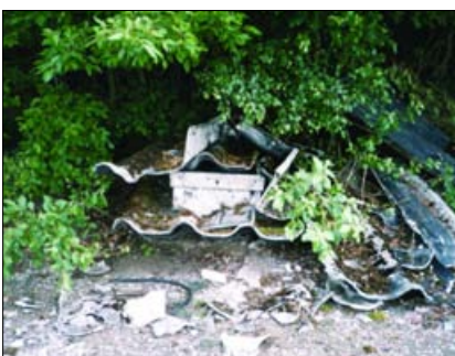
Asbestos cement sheets discarded irresponsibly
